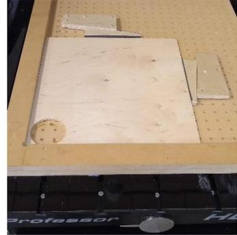
2. Ensure that the correct router bit is installed. 1/8" End Mill.
