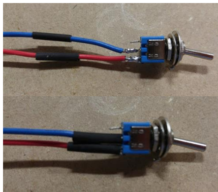
Solder wires to the switch. Notice the heat shrink on the wires first 😊 Make sure you do not burn out the switch by holding the solder pencil TOO LONG on the switch legs.
