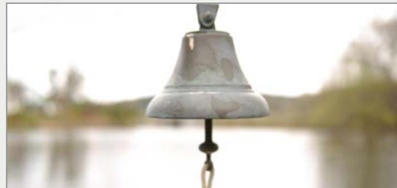
**All boats 12 m (39'4") or more** must have a fitted whistle. Boats over 20 m (65'7") must also have a bell. Check Annex III of the *Collision Regulations* for the technical standards these appliances must meet.
