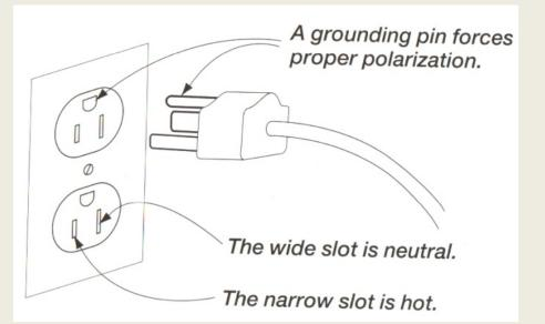
\*\*Proper installation of a receptacle is with the Ground facing down!!
