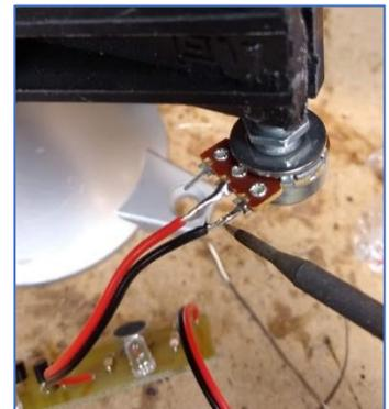
**Step 10** – Solder the other ends of the potentiometer’s wire into the board. It does not matter which wire goes in which hole as potentiometers HAVE NO POLARITY.
