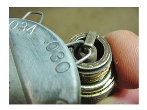
Step 4 - Tap side electrode on solid surface to adjust smaller
