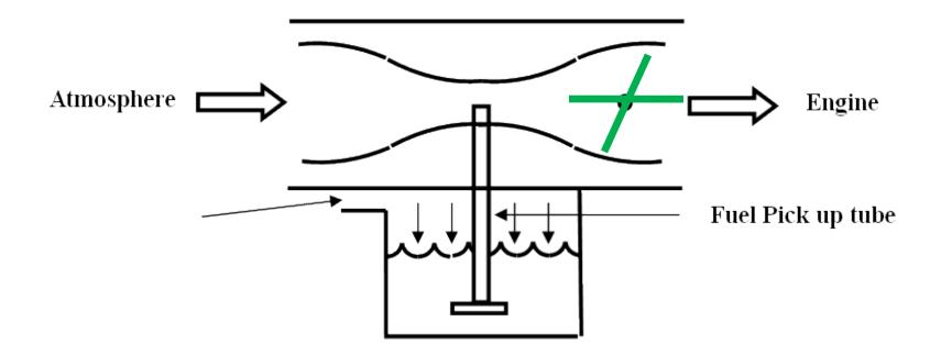
The <u>Throttle Control Lever</u>, is connected to the Throttle Valve and allows you to vary the speed manually (pull/push)
