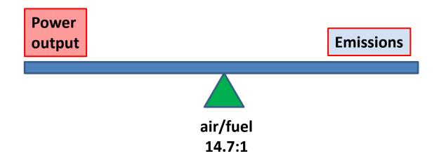
It is possible to mix the air and fuel for better emission, but the result is reduced power output.
