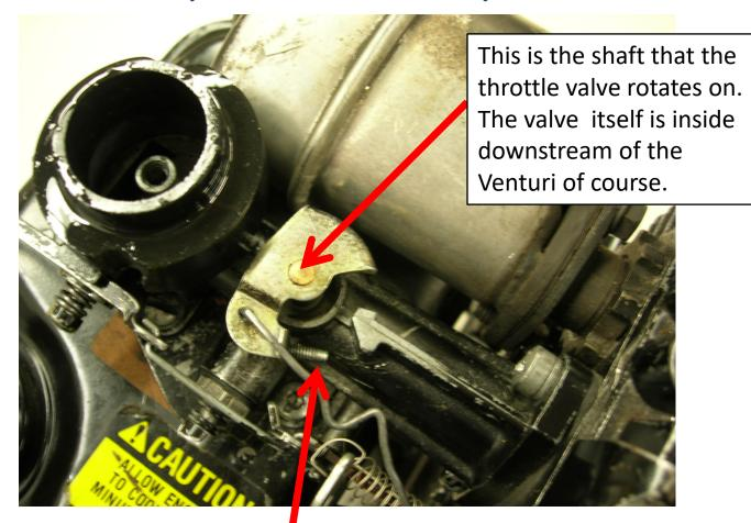
Turning the **Idle Set Screw** opens the throttle valve and speeds up the idle
