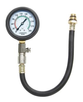
For engines of this type, readings between 40 and 60 psi "generally" indicate good compression.
