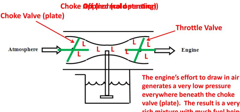
everywhere beneath the choke valve (plate). The result is a very rich mixture with much fuel being pushed up the tube and little air being combined with it.
