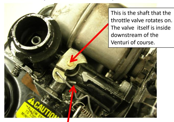
Turning the screw in opens the throttle valve and speeds up the idle
