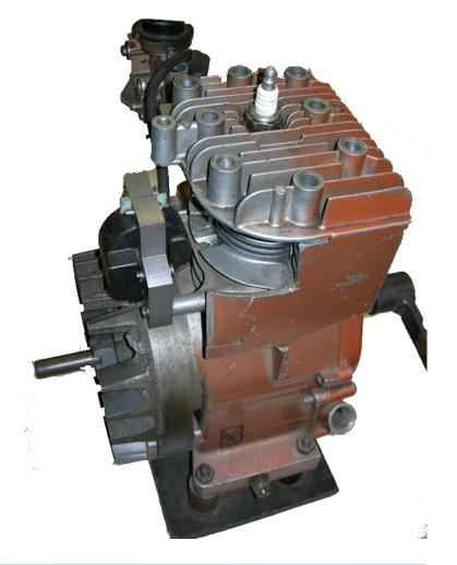
When removing or installing a cylinder head the fasteners must be removed and installed in a 'sequence' as specified by the manufacturer. This is generally called the 'Torque sequence'. HINT: In the book – Section
