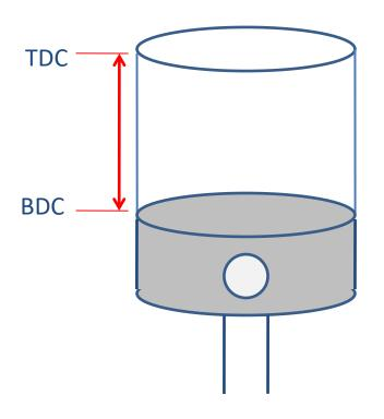
After finding the 'swept volume' for a single piston, we'll multiply this by the number of cylinder's, or pistons, the engine has
