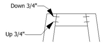
3) Measure up 3/4" or 20mm from the bottom of the rail all the way around the stool - place a pencil mark across the legs and rail as above
