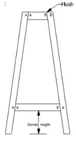
2) With the stool clamped, measure down from the top of the rails 5/8" or 3/4" or 20mm on the outside all the way around the stool - place a pencil mark across the legs and rail
