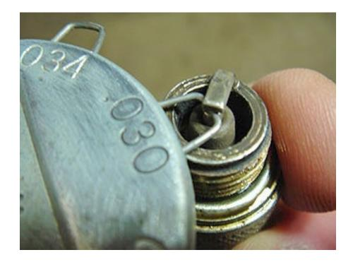
Step 3 - tap side electrode on solid surface to adjust smaller
