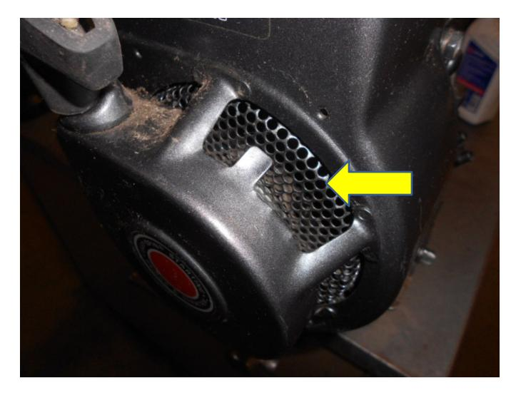
8. Caution: Spinning crankshaft on 'less visible side of engine'.
