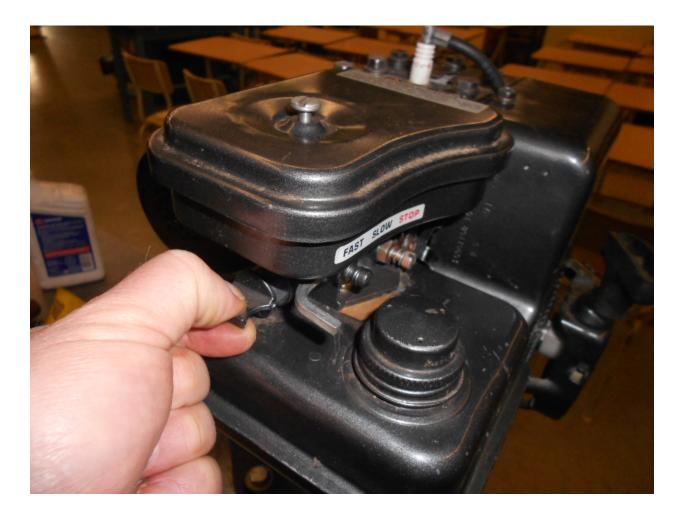
8. Outside, With engine secured in a vise. Use the recoil starter to start the engine.
